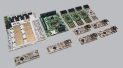
Development modules are available to enable rapid design development. The modules are available in a variety of mechanical formats to allow easy bread-boarding or immediate access to the bridge interfaces. Additionally application modules are available which provide specific system functionality.
