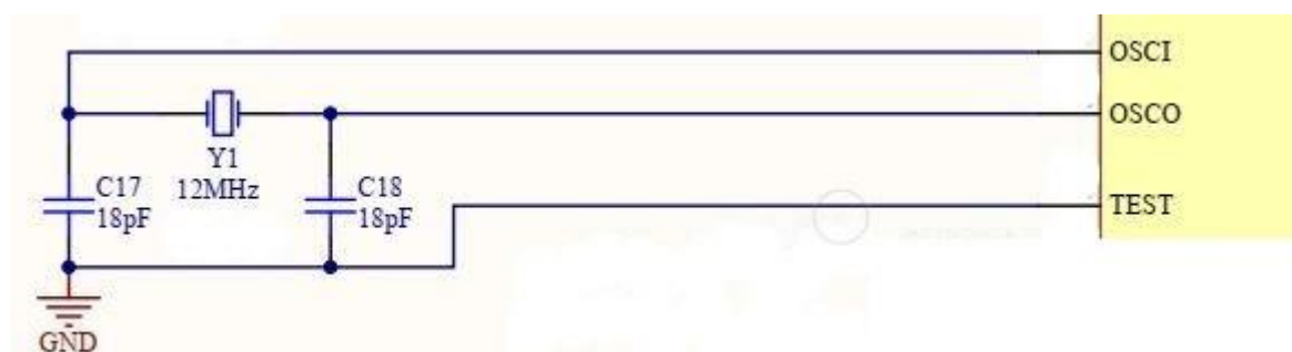
Figure 33 - Recommended FT233HP/FT232HP Crystal Oscillator Configuration
