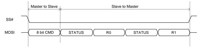
Figure 6.11 Half Duplex 3-pin Data Master Read
