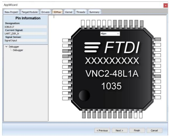
Figure 5.5 VNC2 Toolchain App Wizard showing IOMux Configuration
