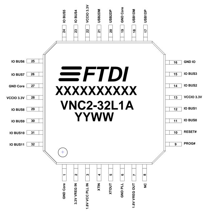
Figure 3.1 32 Pin LQFP – Top Down View
