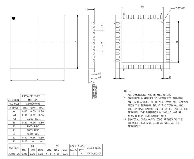
Figure 11. 6 QFN-48 Package Dimensions
