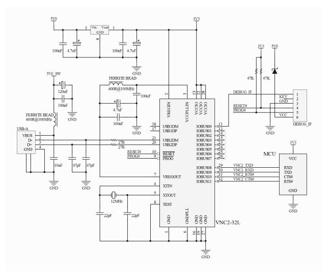
Figure 10.1 VNC2 Schematic (MCU – UART Interface)
