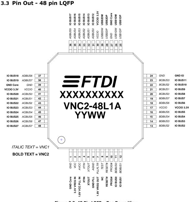
Figure 3.3 48 Pin LQFP – Top Down View
