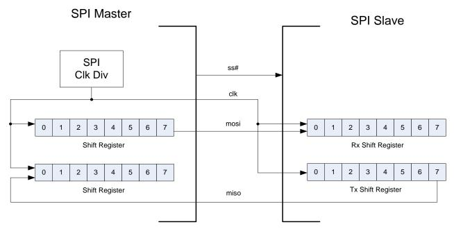
Figure 6.12 Unmanaged Mode Transfer Diagram
