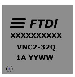
Figure 11.2 Markings – 32 QFN
