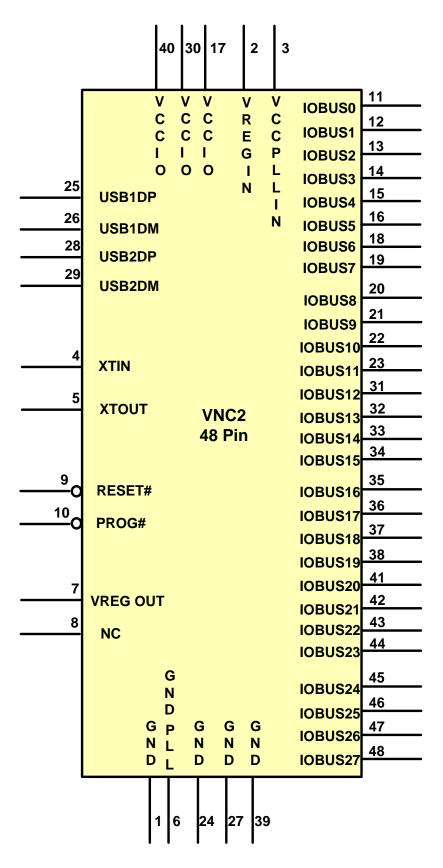
Figure 3.6 Schematic Symbol 48 Pin
