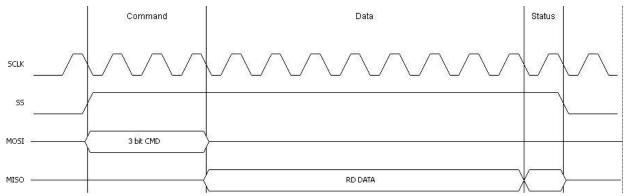
Figure 6.19 SPI Slave Mode Status Read
