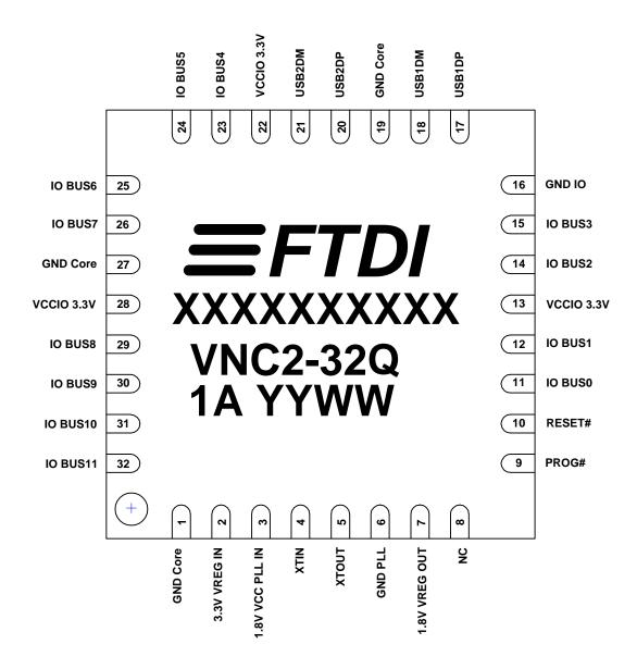
Figure 3.2 32 Pin QFN – Top Down View
