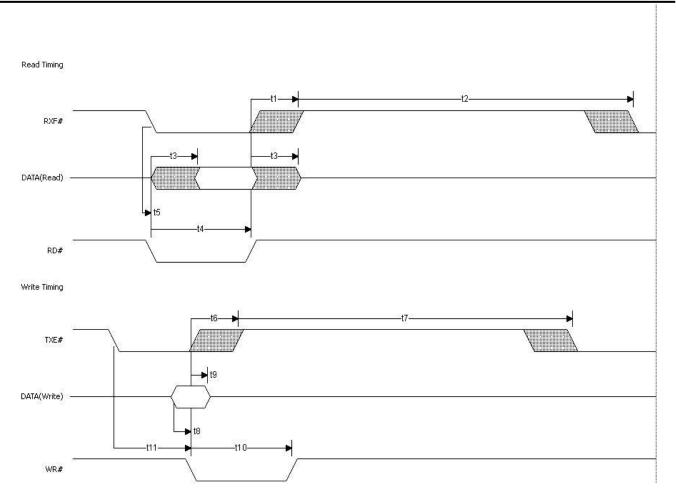
Figure 6.22 Asynchronous FIFO mode Read / Write Cycle
