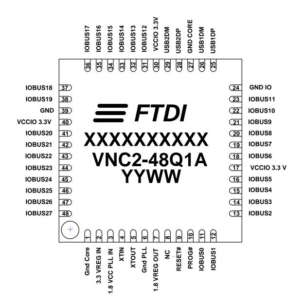
Figure 3.4 48 Pin QFN – Top Down View
