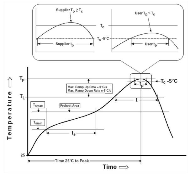
Figure 11.7 All packages Reflow Solder Profile
