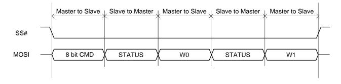
Figure 6.10 Half Duplex 3-pin Data Master Write
