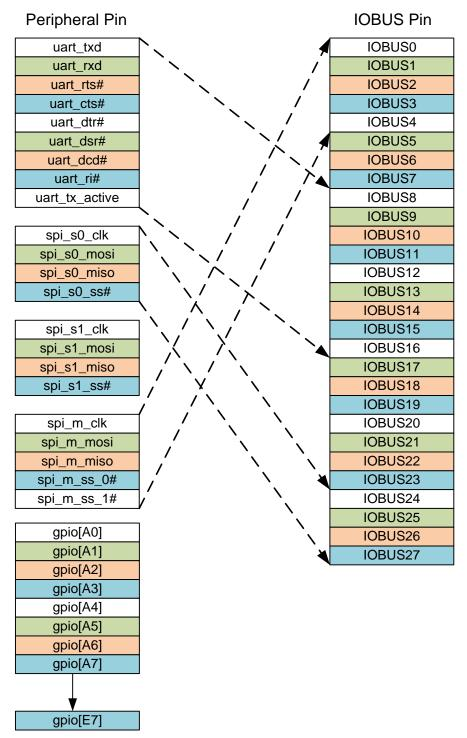
Figure 5.3 IOBUS to UART, SPI slave0 and SPI master second example
