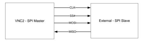
Figure 6.20 SPI Master block diagram
