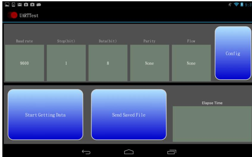
**Figure 3.10 UART Test Application Screen**
