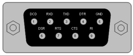
Figure 3-1 RS232 DB9 Pin Out
