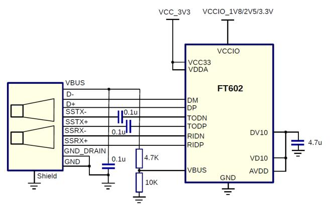
Figure 6.2 Self-Powered Configuration
