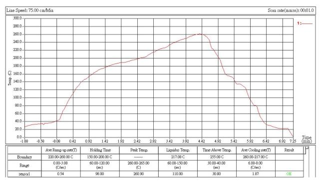
Figure 8.3 Solder Reflow Profile
