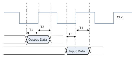
Figure 4.4 FIFO Bus AC timing diagram
