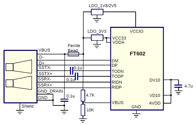
Figure 6.1 Bus-Powered Configuration-1.8V/2.5V I/O
