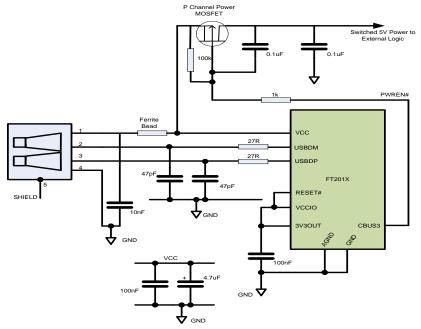
Figure 7.3 Bus Powered with Power Switching Configuration
