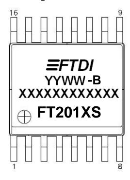
Figure 11.2 SSOP-16 Package Markings
