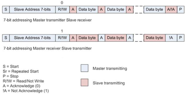
Figure 9.1 Data transfers using 7-bit addressing
