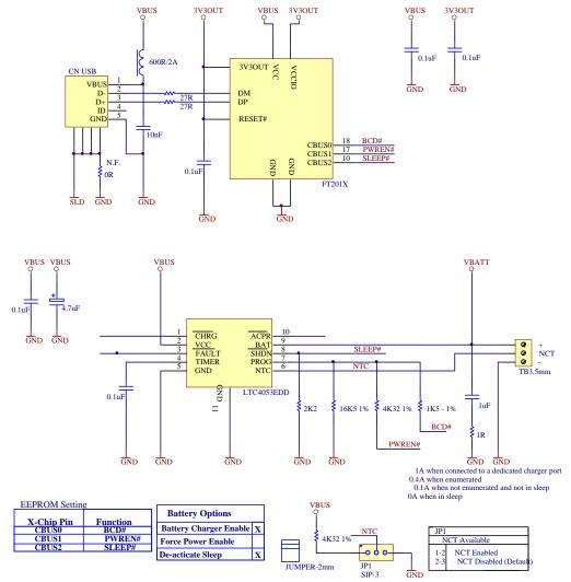
Figure 8.4 USB Battery Charging Detection (3 - pin)
