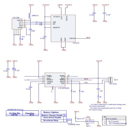
Figure 8.2 USB Battery Charging Detection (1- pin)
