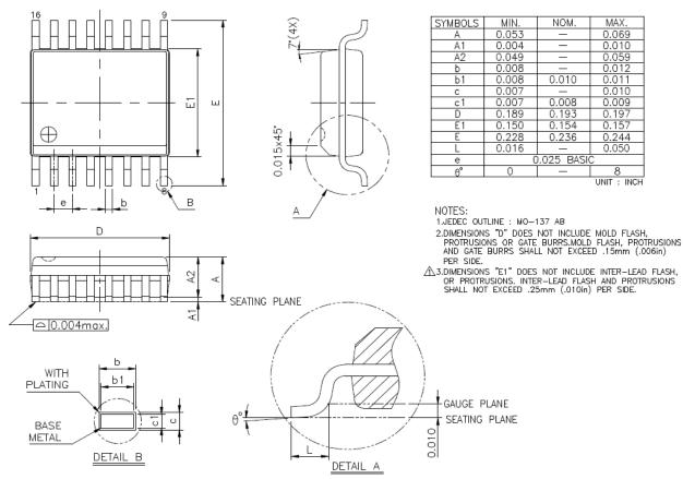
Figure 11.1 SSOP-16 Package Dimensions
