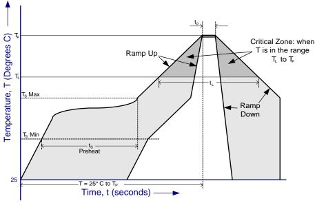
Figure 11.5 FT201X Solder Reflow Profile
