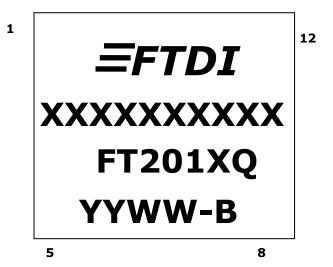
Figure 11.4 QFN-16 Package Markings
