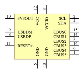
Figure 3.2 SSOP Schematic Symbol
