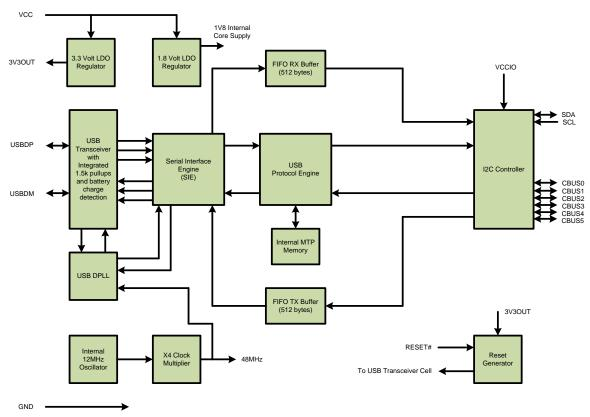
Figure 2.1 FT201X Block Diagram
