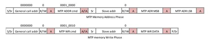
Figure 10.2 Write EEPROM command sequence
