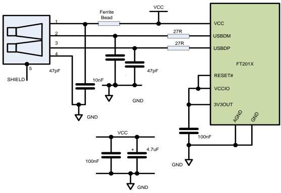
Figure 7.1 Bus Powered Configuration
