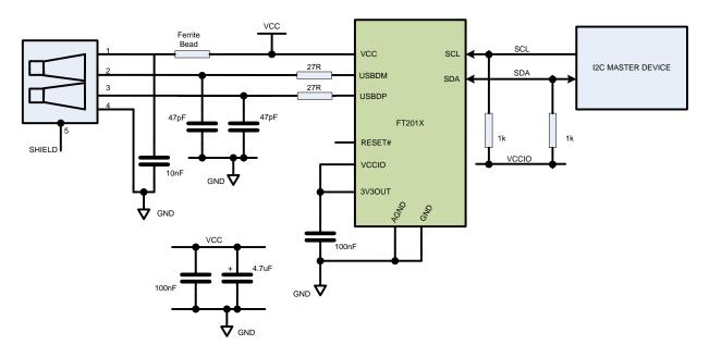
Figure 8.1 Application Example showing USB to I<sup>2</sup>C Converter
