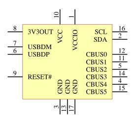
Figure 3.1 QFN Schematic Symbol
