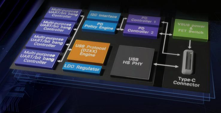
The Power Delivery series has up to two Type-C/PD ports, with PD1 port supporting both power sink and source roles (Initial Sink), and PD2 port only supporting a power sink port role.
