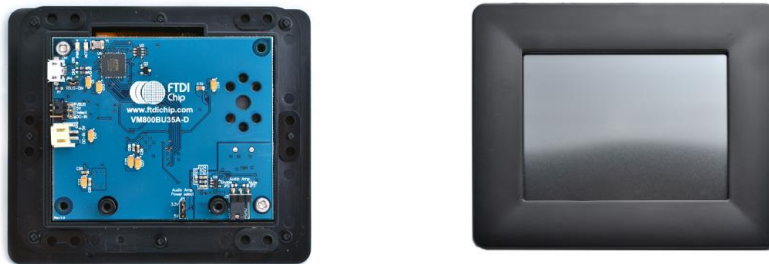
Figure 3-1 - VM800BU module profile 3.5" display version
