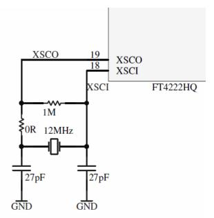
Figure 7.4 Recommended FT4222H Crystal Oscillator Configuration
