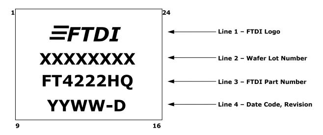
Figure 10.2 VQFN-32 Package Markings
