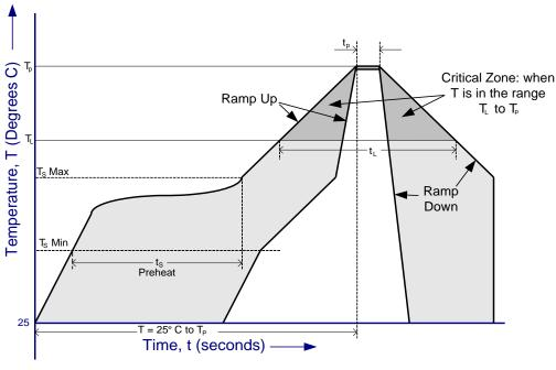
Figure 10.3 FT4222H Solder Reflow Profile
