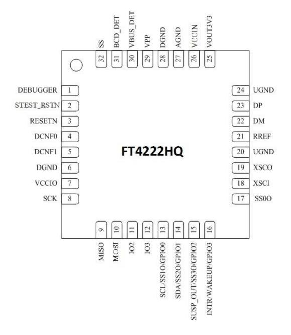
Figure 3.1 Pin Configuration VQFN-32 (Top-Down View)
