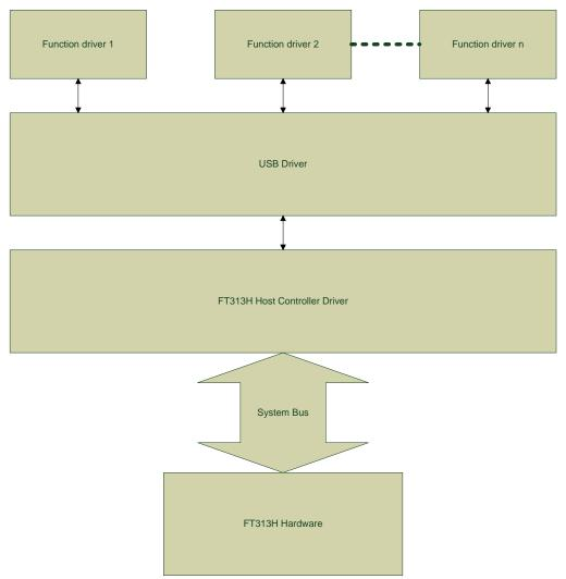
Figure 1: USB host software architecture
