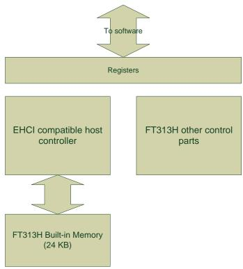
Figure 2: Block diagram of FT313H
