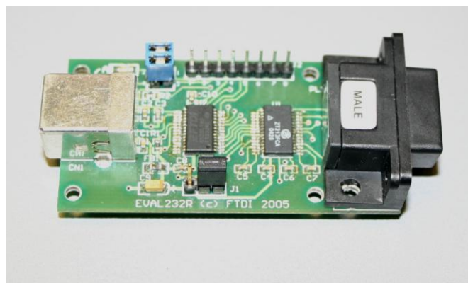
Fig. 2 – EVAL232R with a DB9-RS232-USB-M
