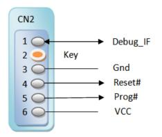
Figure 2.2 VNC2 Debugger/Programmer Module Connector
