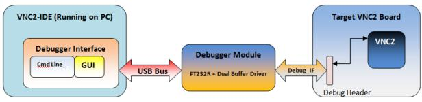
Figure 2.1 VNC2 Debugger Interface
