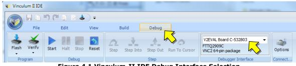
Figure 4.1 Vinculum-II IDE Debug Interface Selection
