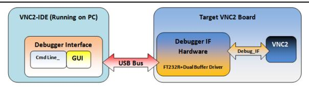
Figure 2.3 Debugger Interface on Target VNC2 Board
