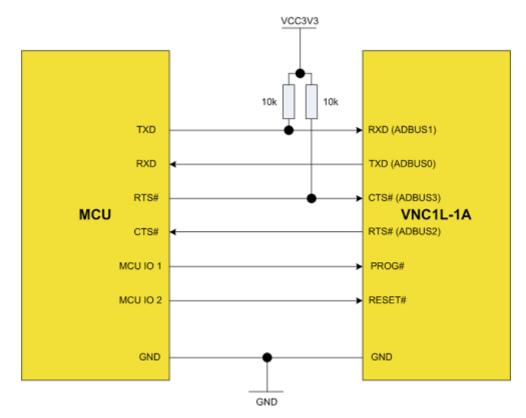
To enable the bootloader, the PROG# pin must be driven low and the VNC1L must then be reset by driving the RESET# pin low then high. Run mode can be enabled by driving the PROG# pin high and then resetting the VNC1L by driving the RESET# pin low then high.
