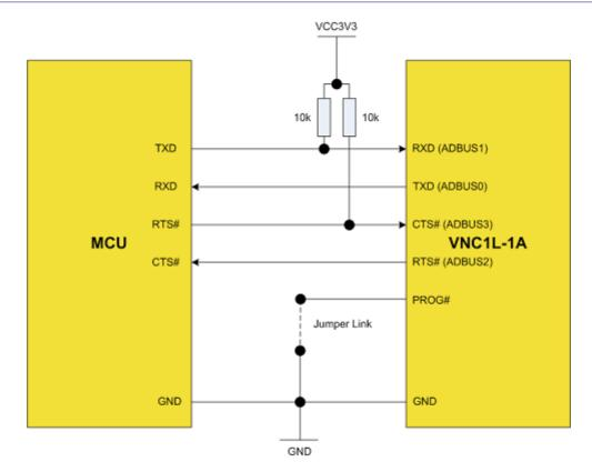
Note that for the bootloader to be active the jumper must be fitted before powering the VNC1L. If the jumper is not fitted, the VNC1L will power up in run mode with the bootloader inactive.
