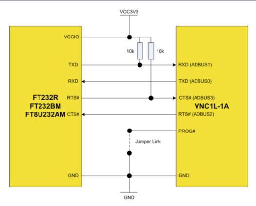
Note that for the bootloader to be active the jumper must be fitted before powering the VNC1L. If the jumper is not fitted, the VNC1L will power up in run mode with the bootloader inactive.
