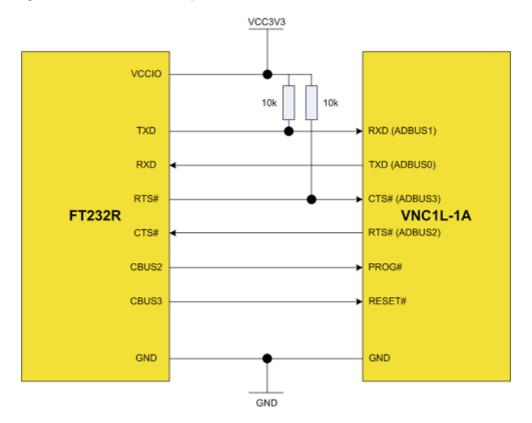
Note that CBUS Bit Bang mode must be enabled in the FT232R EEPROM for CBUS2 and CBUS3 for this to function (see <u>AN232R-01 Bit Bang Modes for the FT232R and FT245R</u> for details of CBUS Bit Bang mode). To enable the bootloader, the PROG# pin must be driven low and the VNC1L must then be reset by driving the RESET# pin low then high. Run mode can be enabled by driving the PROG# pin high and then resetting the VNC1L by driving the RESET# pin low then high.
