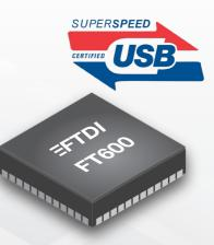
FTDI Chip is proud to announce its first SuperSpeed series in the FT60X, a sophisticated USB3.0 to FIFO bridge in a low count pin package.
