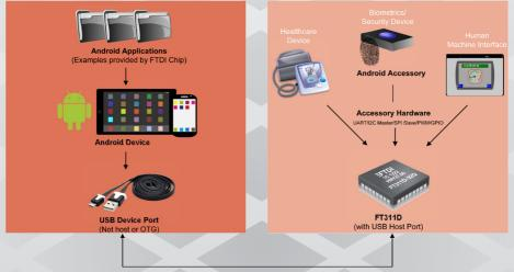
USB Connection providing data connectivity (Optionally, the Android Accessory can also charge the Android device)
