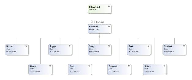
Figure 3.4 Class diagram of the Co-Processor Graphics Library
