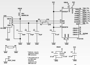
It is possible for the design to simply use RXD and TXD signals but with FTDI solutions the option to implement full modem control is also provided.
