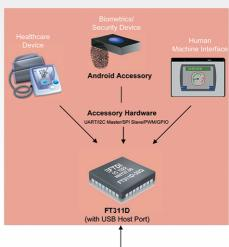
USB Connection providing data connectivity (Optionally, the Android Accessory can also charge the Android device)
