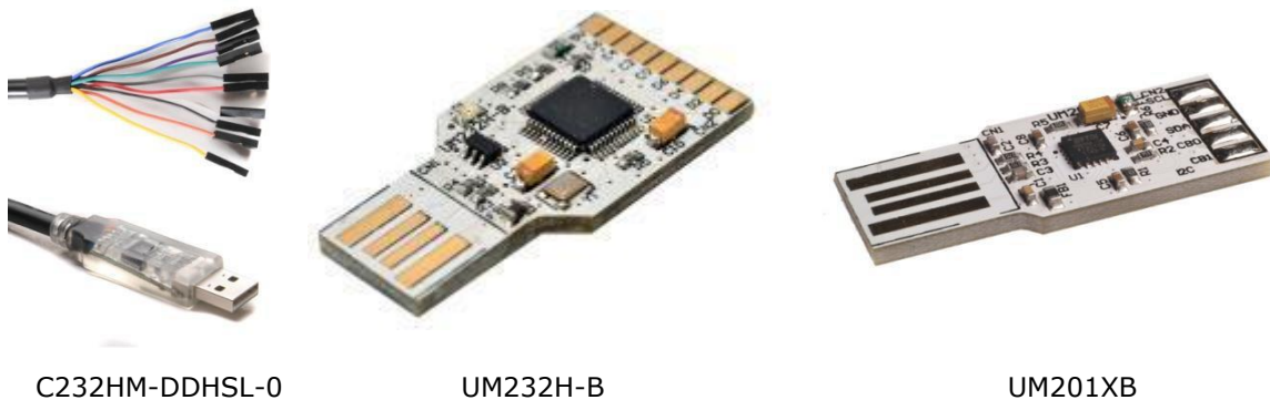
Figure 5.2 Some of the FT232H and FT201X development modules available
